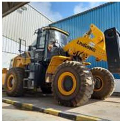
Gambar 1. *Wheel loader* Liugong ZL50CN
